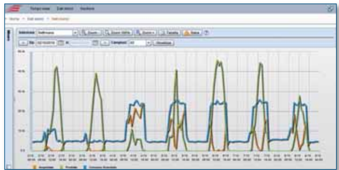
Energy captured, produced and consumed in Energy Sentinel PV.
