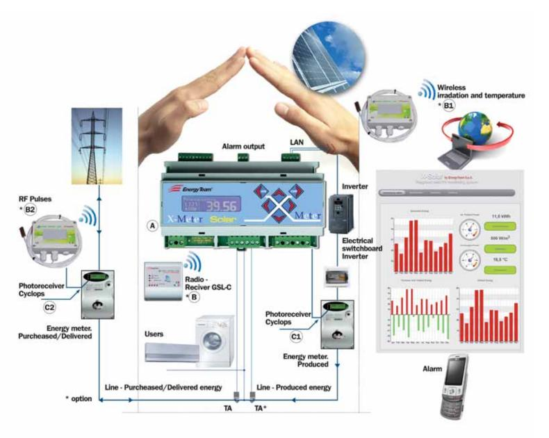
In order to get the maximum control in the performance of the plant, it's possible to insert into the system a combined sensor for Irradiation and panel Temperature, provided by the option for sending data viaradio, useful when the cable installation is difficult.
